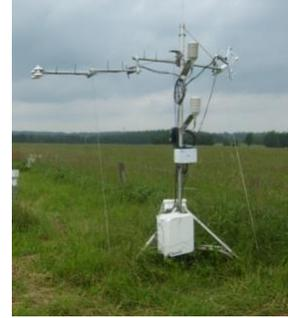
*Atmospheric flux measurements*
